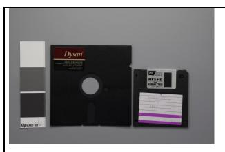
Images above showcase a 5.25-inch floppy disk without sleeve, with sleeve and in comparison to a 3.5-inch floppy disk.
